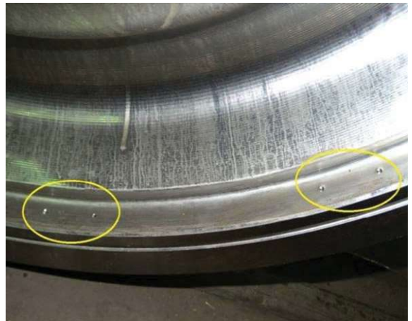
b) Marks left by lathe chuck jaws
