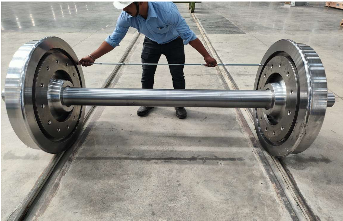
Measured with Mitutoyo make Stick Micrometer (137-204)
